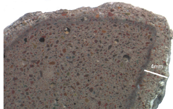
Figure 2 Borax slag cement paste after three months reaction with synthetic leachate
