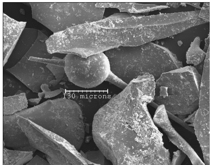
Figure 7 Ferrosilicate slag particles, as supplied. SEM secondary electron image
