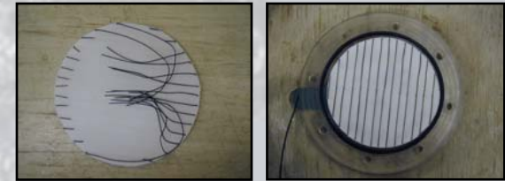
Electrode Preparation - In order to form an electrode system, titanium wires 0.7 mm in diameter, were fixed equidistantly onto a 2 mm thick polyester woven geosynthetic (141 mm in diameter). The ends of each wire were folded behind the filter cloth, joined and then connected to an insulated copper wire leading to the power supply.
